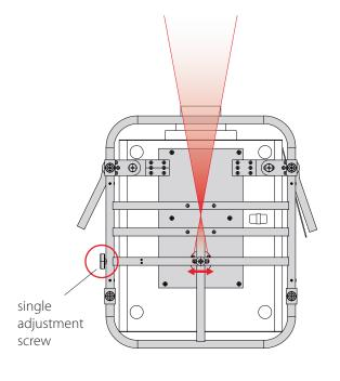
By turning the single round adjustment screw, placed on the side of the frame, you can move the back of the projector to the left or to the right by approximately five degrees.
