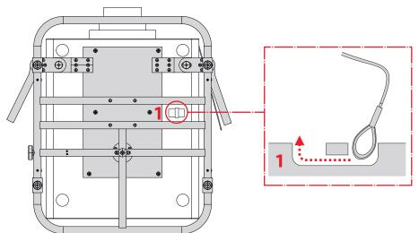
Please use the enclosed steel wire to secure the projector in the frame by drawing the wire around the securing bar (1) of the projector as shown in image 1.
