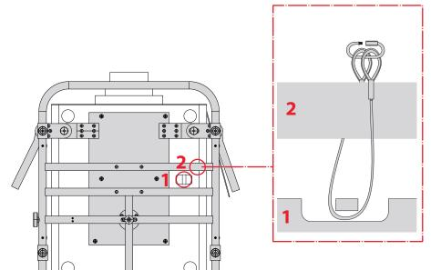
Fix both end latches with the enclosed carabiner. Please make sure that the steel wire clasps the securing bar of the projector (1) and the steel bar of the frame (2). The carabiner screw must be tightly fastened!
