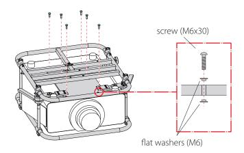
Place the frame on the projector so that it is aligned with the screw hole positions. (Make sure that the forward/back direction is correct when installing. If the direction is reversed, the hole positions will not match up.)
