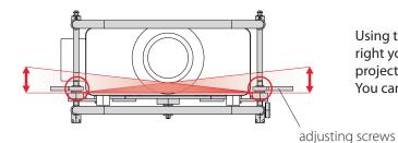
Using the adjusting screws to the left and right you can adjust the position of the projector by approximately five degrees. You can lower or lift the front left or right corner.
